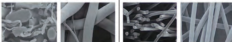
High basis weight meltblown: similar to depth effect increases dust holding capacity
