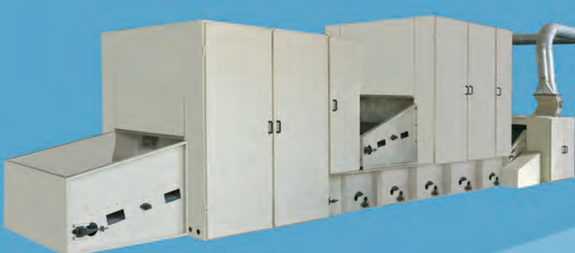
直列式混开棉机组 In-line mixing opener
